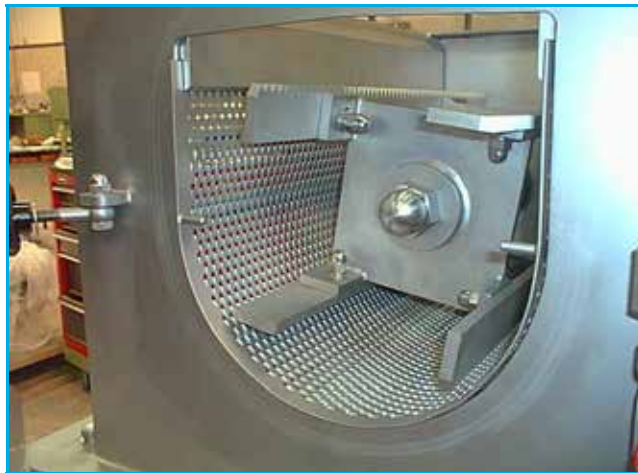
Internal view of Kemutec Kibbler, with Cantilever Shaft
