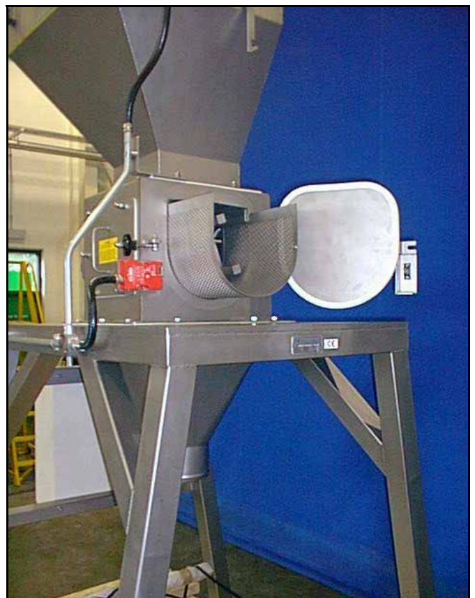
Kemutec Kibbler showing Hinged End Door and Screen partially removed
